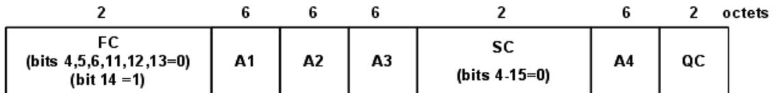
**Figure 43p—AAD construction**
