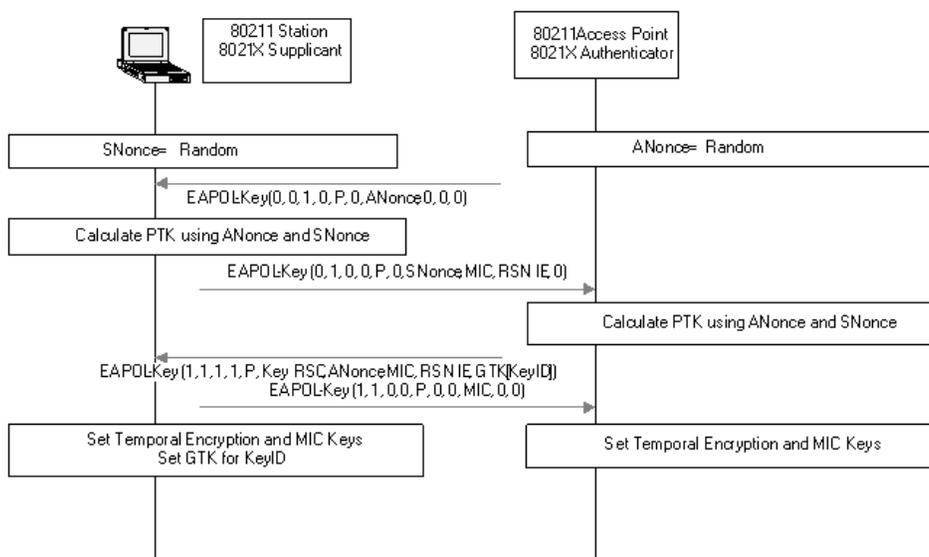
**Figure 43ac—Sample 4-Way Handshake**
