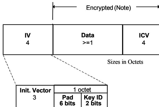
NOTE—The encipherment process has expanded the original MSDU by 8 octets, 4 for the IV field and 4 for the ICV field. The ICV is calculated on the Data field only.
