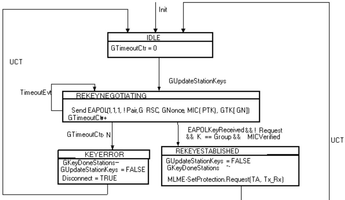
Figure 43ah—Authenticator state machines, part 3
